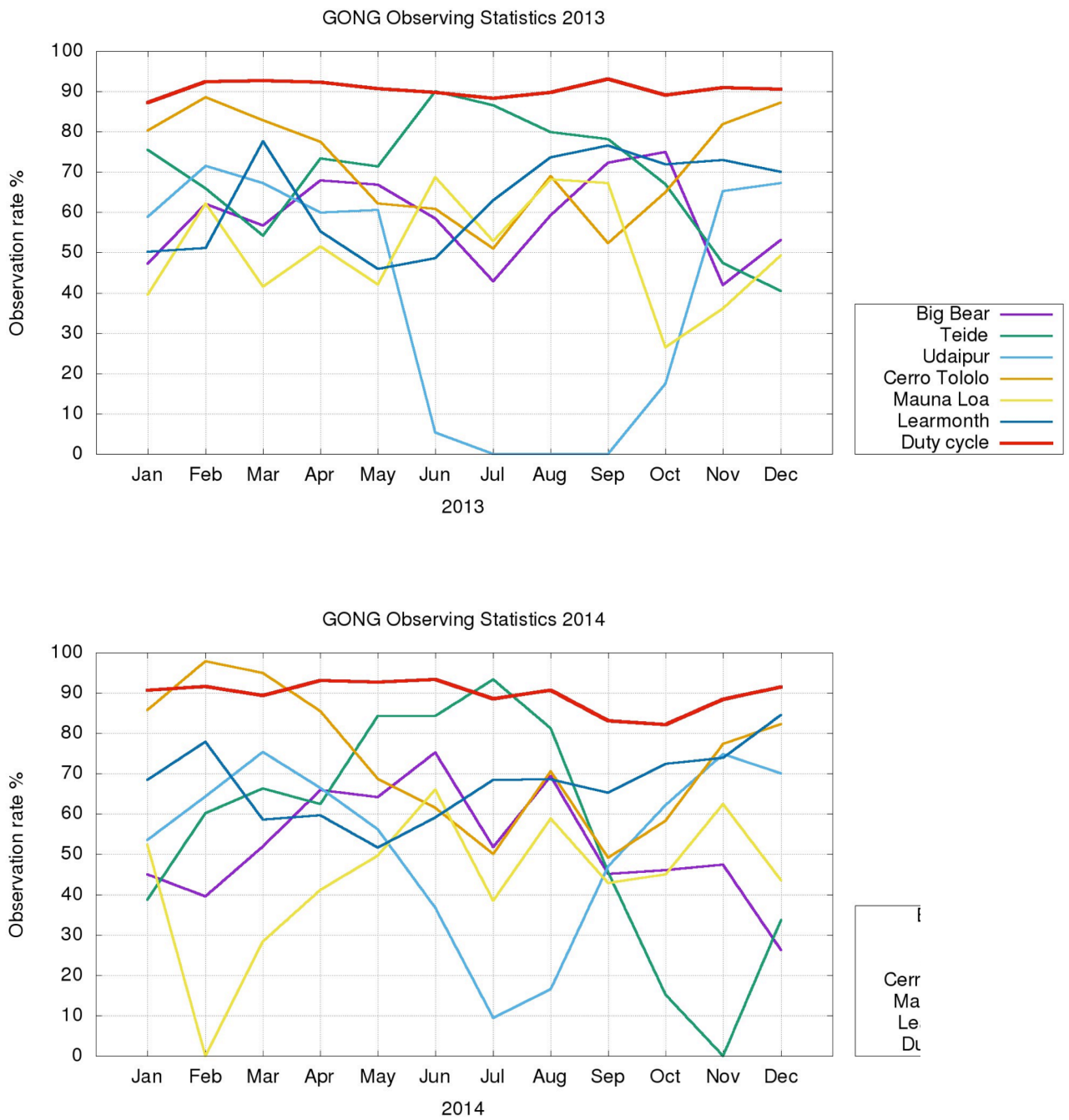
Figure 6.1: Duty cycle (red) and percentage of possible observing time for the six GONG sites for the years 2013 and 2014.
