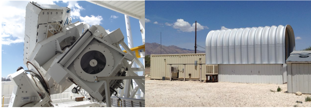
Figure 4.4: Left panel shows SOLIS, a 50 cm aperture full-disk telescope mounted on an equatorial mount. Right panel shows the retractable dome that covers SOLIS.
