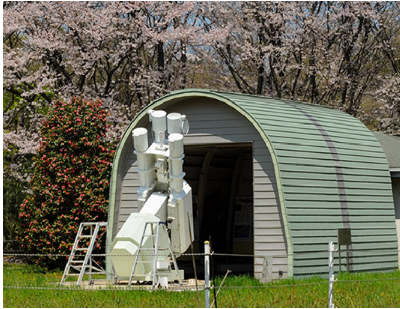
Figure 4.6: The Solar Flare Telescope at Mitaka, NAOJ, Japan, is a combination of four parallel full disk telescopes performing (i) H-alpha and white-light imaging, (ii) infrared spectropolarimetry, (ii) G-band imager, and (iv) white light imager.
