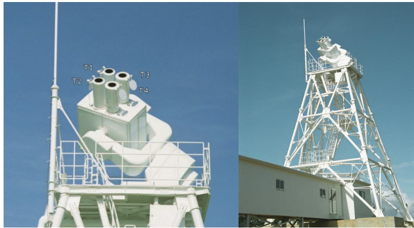
Figure 4.5: Solar Magnetic Activity Research Telescope (SMART), Hida Observatory, Kyoto, Japan. It is a combination of four parallel telescopes, two performing full-disk H-alpha imaging and vector magnetography in the Fe I 630.2nm spectral line, and two telescopes performing high resolution (limited FOV) observations in 630.2 (vector magnetography) and H-alpha (core and wing emission).
