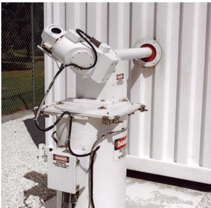
Figure 4.3 GONG turret system connected to shipping container which houses the instrument.
