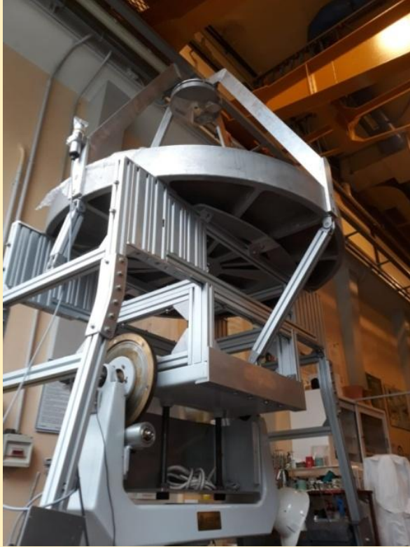
SOLARIS antenna opto-mechanical components
