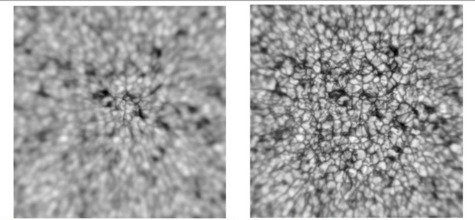
Conventional (left) and multi-conjugate (right) solar adaptive optics (Schmidt et al., Astron. Astrophys. 597, L8, 2017). Conventional AO produces a sharp image only at the center of the field, limited to a single isoplanatic patch of 5 arcsec. MCAO extends the compensated field to 30 arcsec with three deformable mirrors in this case.
