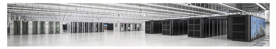
Piz Daint is a Cray HPC system located at CSCS in Lugano, consisting of XC50: *5704 hybrid nodes* of 12 cores with Nvidia Tesla accelerators and 64GB RAM, and XC40: *1813 multicore nodes* of 2 x 18 cores with 64/128 GB RAM. Intel Xeon E5 CPUs.
