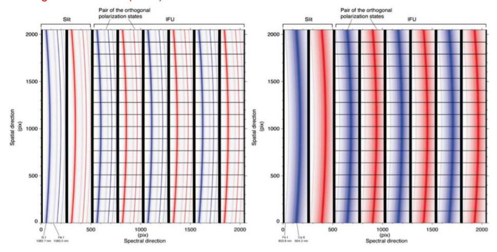
Simulated spectra on the detector for He I 1083 nm (left) and for Ca II 854 nm (right).
