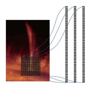
Concept of an *optical fiber IFU*. The 2-D array of the optical fibers at the entrance of the IFU (left) is converted into 3 arrays (slits) at the exit of IFU (right), which feeds the light into the spectrograph.
