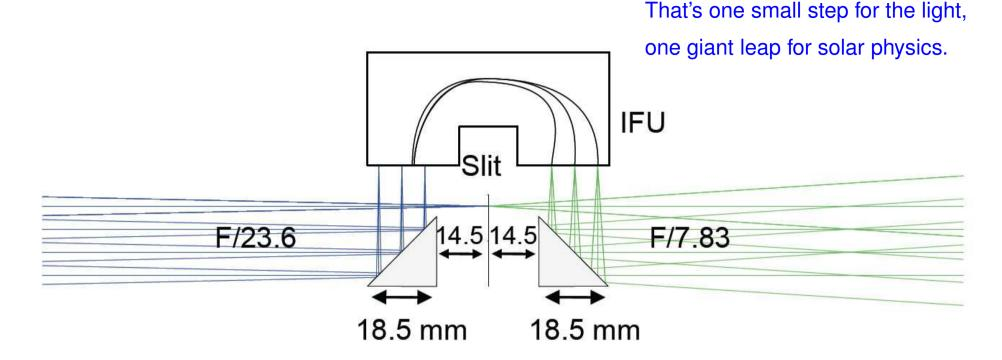
The IFU injects lights from the 3 slits into the spectrograph while the true single slit also injects light simultaneously. In total *4 spectra are created* at the spectrum mask.
