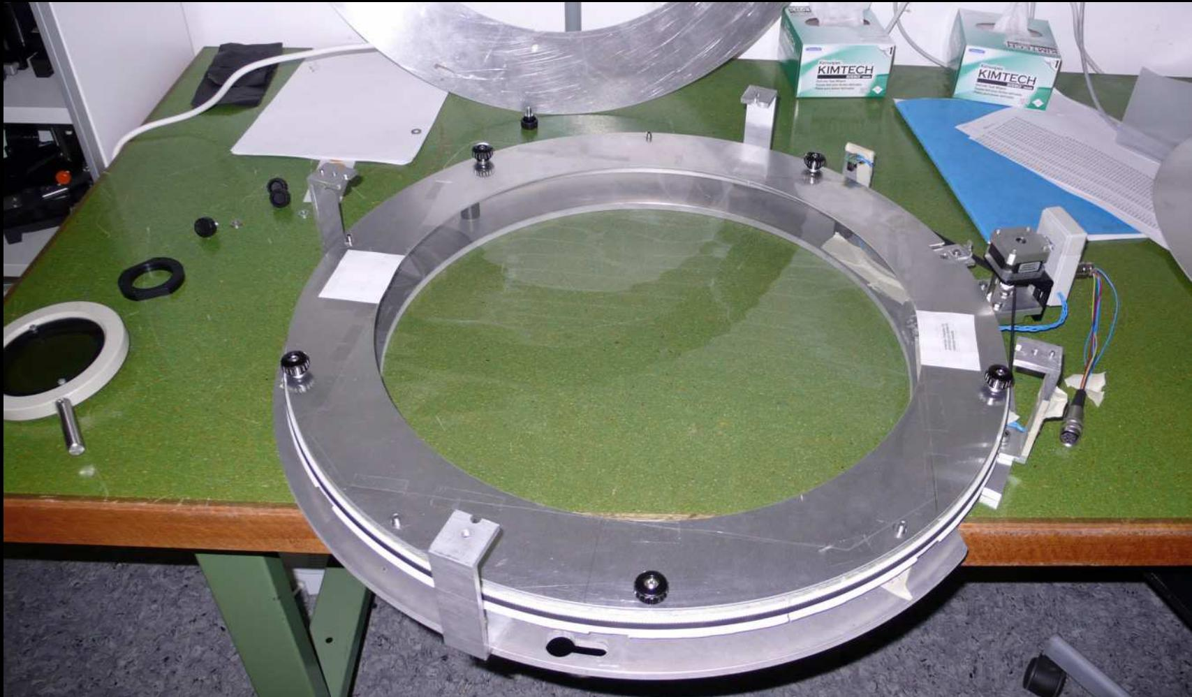
Zero order half wave retarder film mounted on a motorized rotatable circular flange.
