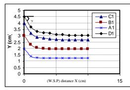
**Figure 5.** (W.S.P) for gate inclined  $(\beta=45)^{\circ}$  in the direction of flow with sharp edge  $(\theta=45)^{\circ}$ .
