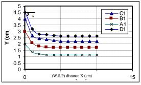
Figure 7. (W.S.P) for gate inclined ( $\beta$ =45)<sup>o</sup> opposite the flow direction with sharp edge ( $\theta$ =45)<sup>o</sup>
