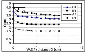
**Figure 4**. (W.S.P) for gate inclined  $(\beta=45)^{\circ}$  in the direction of flow with horizontal edge  $(\theta=0)^{\circ}$ .
