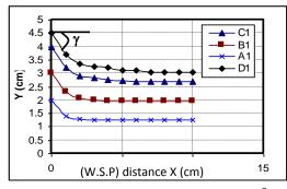
**Figure 3.** (W.S.P) for the vertical gate  $(\beta=0)^{\circ}$  with horizontal edge  $(\theta=0)^{\circ}$  (Where (x) is the horizontal distance of (W.S.P) from the sluice gate, and (y) is the vertical distance (depth) of (W.S.P) from channel bed to sluice gate opening)
