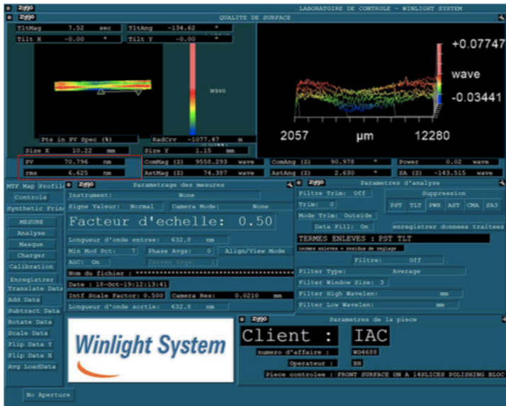
Flatness measurement of a stack of 14 slices – full aperture
